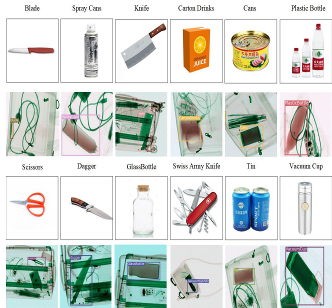
Fig. 1. Samples of 12 categories and corresponding X-ray images. The X-ray image dataset contains various cutters and liquid containers that may contain flammable or explosive liquids.
